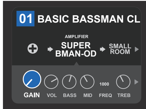
Close-up detail of the CONTROLS LAYER, in which the gain control for the amp model within the preset is selected.
