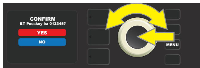
When first pairing a Bluetooth device with Rumble Studio 40/Stage 800, an onscreen prompt in the amplifier’s DISPLAY WINDOW will ask for pairing verification; use the ENCODER to scroll to and select either “YES” or “NO.”
