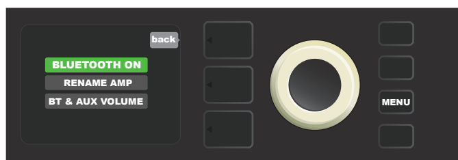
The amp’s default Bluetooth function is “ON” (as labeled in green box); select “RUMBLE” on external device.
