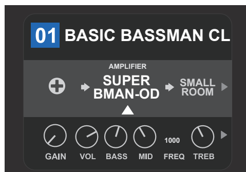
The amp model within the preset is selected here in the SIGNAL PATH LAYER, as indicated by the white arrow and the word “amplifier.” It is flanked by one occupied effect slot (right) and one empty effects slot (left).
