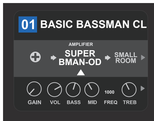
Close-up detail of a different preset that includes an open slot in which an effect can be placed, marked here by a placeholder symbol (a plus sign in a circle) at the far left end of the SIGNAL PATH LAYER.
